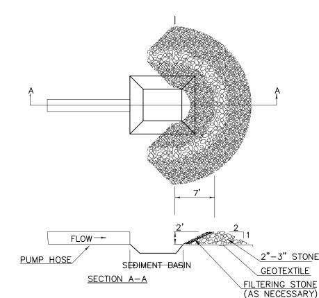
TEMPORARY DEWATERING NOTES: LOCATIONS OF COFFERDAMS AND WATER DIVERSION COMPONENTS DETAILED ON THE PLANS ARE APPROXIMATE AND MAY BE ADJUSTED AS REQUIRED TO ACCOMMODATE THE
